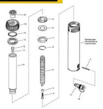
Enerpac RC2510K - Kit for Single Acting CylindersThe Enerpac RC2510K is a kit for the singleacting cylinders (RC-series and equivalent).
