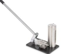
Enerpac ultra-high-pressure, hydraulic hand pumps are offered as single-stage or 2 stage manual pumps that can handle up to 40,000 psi (2800 bar). Typical industrial applications include lifting, testing, calibration, maintenance, and repair. The P2282 m
