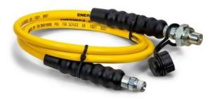
H700-Series Hoses have a safety factor of 4:1 to provide the reassurance and reliability needed for demanding high-pressure applications. Each hose contains two layers of steel wire braids covered by a polyurethane sleeve - providing the strength and ab
